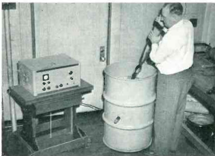
Instrument at left rings bell and lights lamp when heat-treated steel part has been quenched sufficiently in cold water
