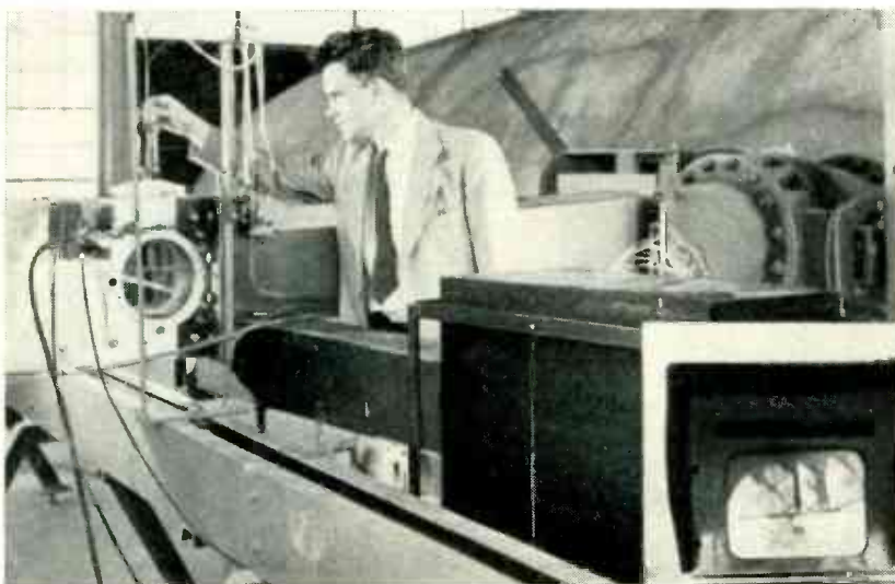
Television camera at Lewis Flight Propulsion Laboratory views the test section of a small supersonic wind tunnel. Insert at lower right shows the received Schlieren image of the test section showing the shock pattern
