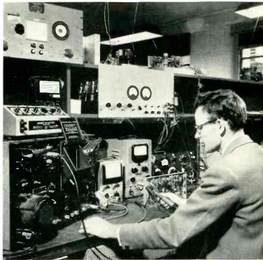
Complete bench test set-up at The Glenn L. Martin Co. plant in Baltimore for testing advanced fire control systems for aircraft turrets. Major components of a modern system include (1) sighting system for determining direction and distance of target, (2) computing mechanism for determining where to point guns so bullets will hit target, and (3) motor-driven mechanisms for moving turret and guns and for supplying ammunition. In the more advanced modern systems the operator need only select his target on a radar screen and fire the guns when the target comes into range
