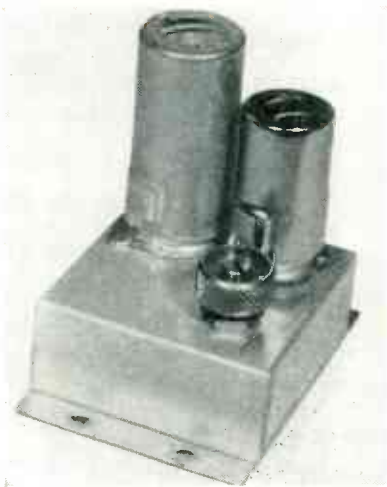
Master pulse generator operates the ring-of-8 counter chain
