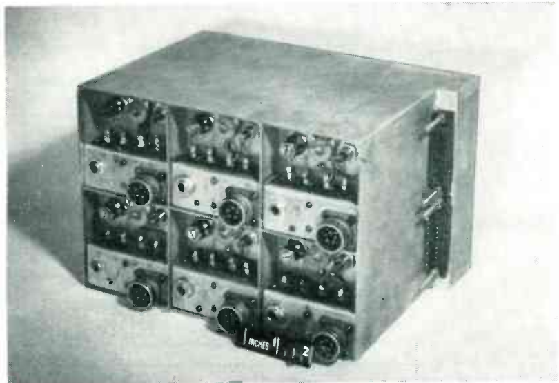
Front of six-channel amplifier, showing size relative to rule at lower right
