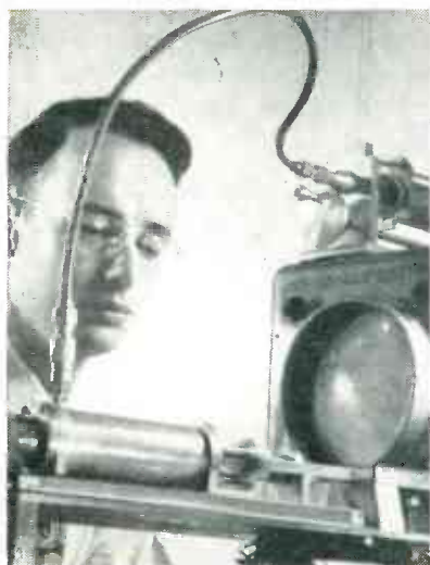
Microwave sweep generator facilitates adjustment of matching between wide-band tubes and transmission lines
