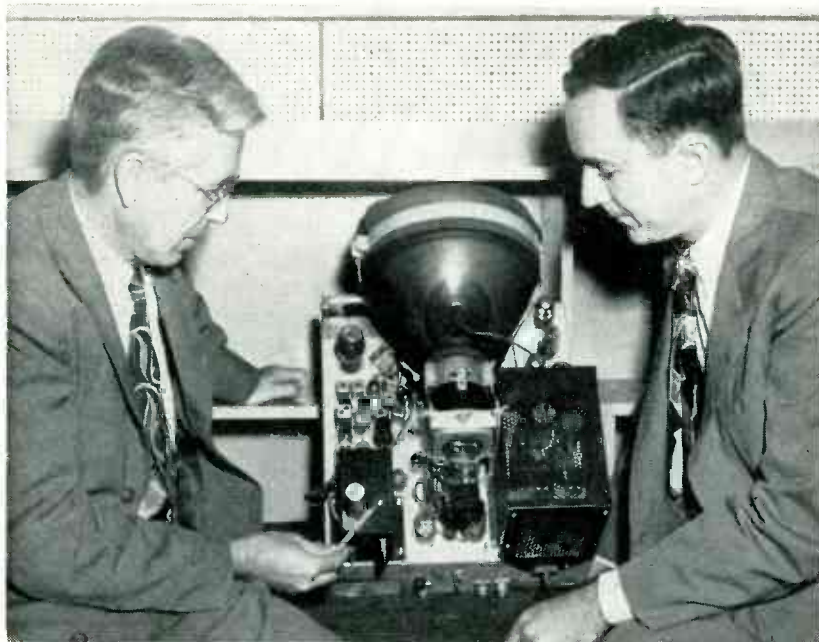
Chapin and Roberts, of FCC staff, point to automatic bracket-standard switch they developed and installed on Bendix model 235M1 chassis
