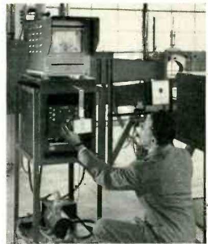
Engineer checks test pattern on portable monitor. Camera, below monitor, is mounted in acoustic shield
